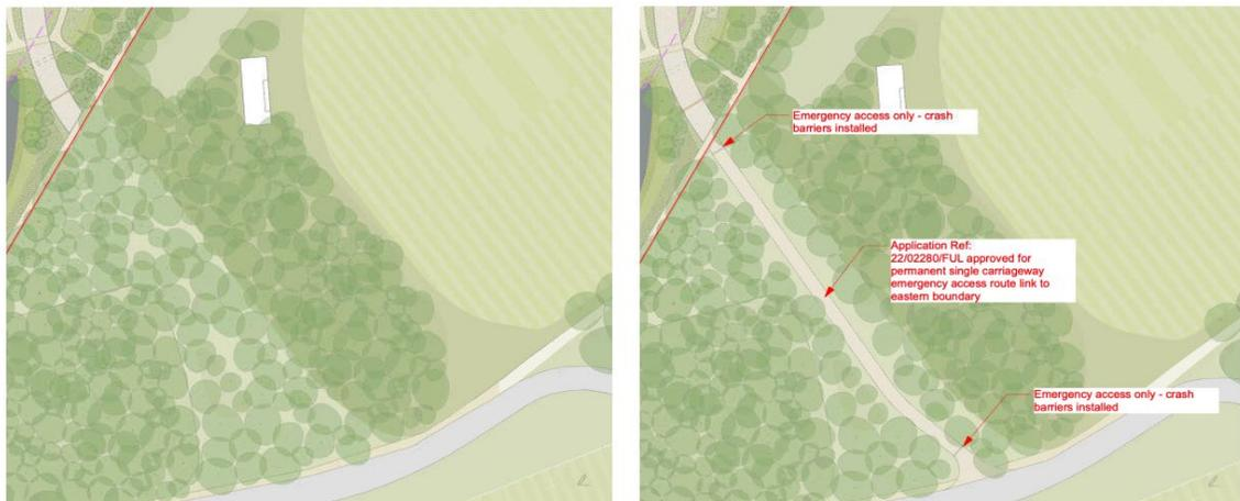
**Figure 4: Addition of emergency access (TCAR2)**
