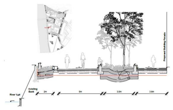
Figure 5: proposed section of the riverside walkway
