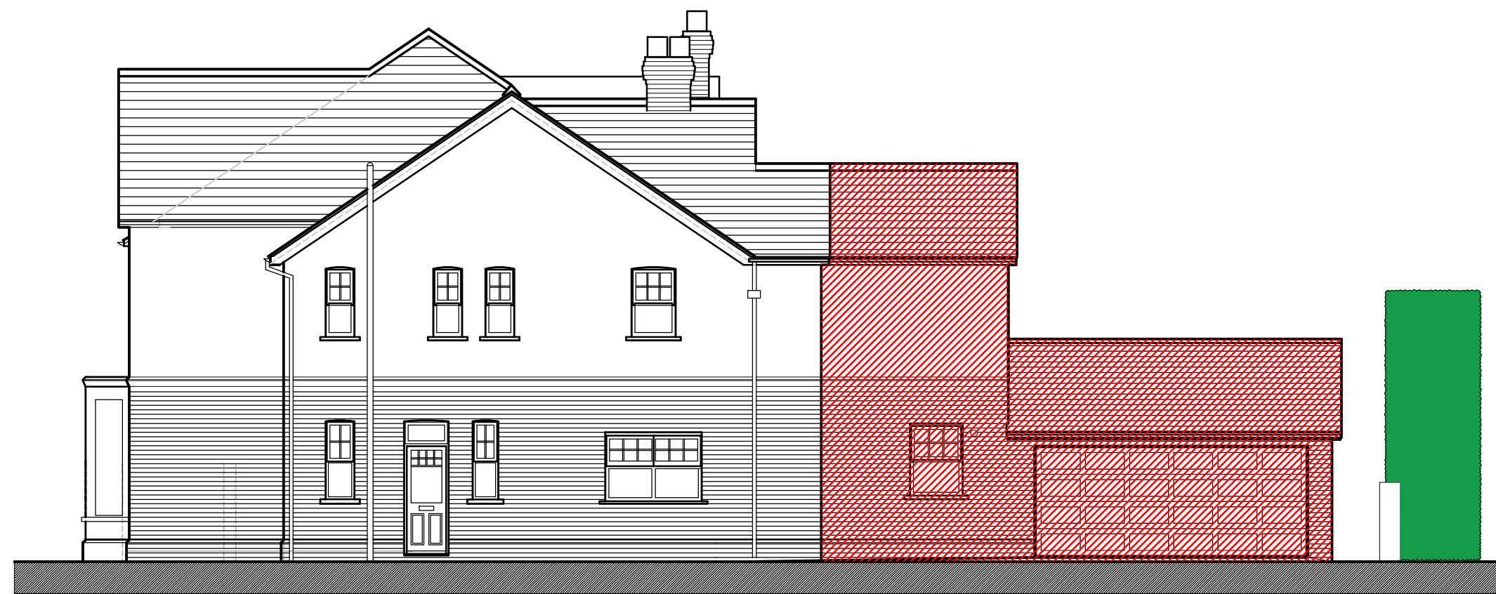
Existing Elevation to Westbourne Crescent Showing Demolitions
