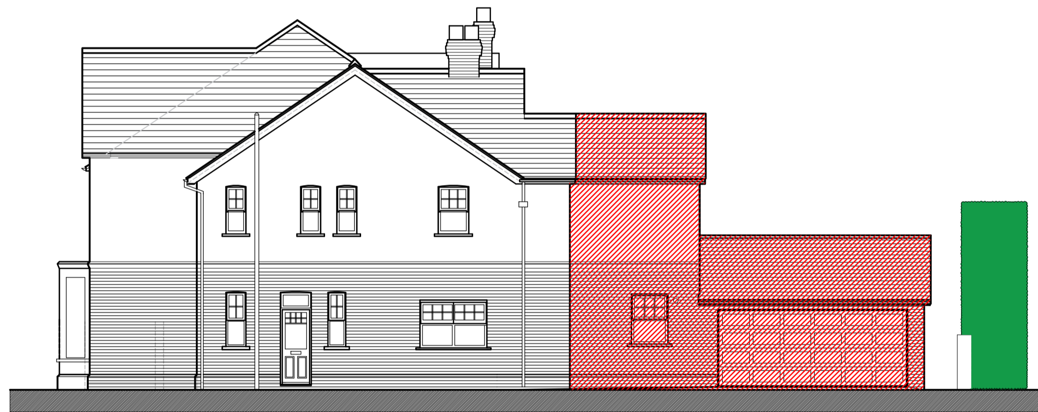
Existing Elevation to Westbourne Crescent Showing Demolitions
