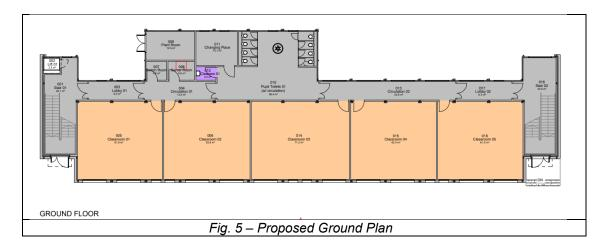
3.4 The building would be of contemporary appearance comprising a simple box form, with a flat roof, being clad in brickwork from ground to ground floor window head height and aluminium cladding panels, in a 'Pearl Mouse Grey' to upper storey.
